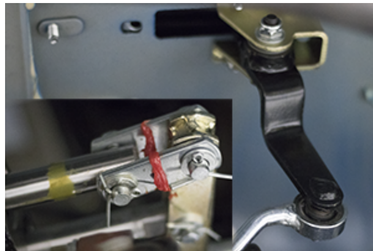
Figure 18. Shift Linkage Pivot Points
