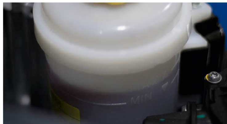
Figure 14. Power Steering Fluid Level
