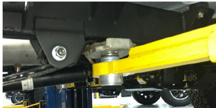
Figure 7. Rear Lifting Location
