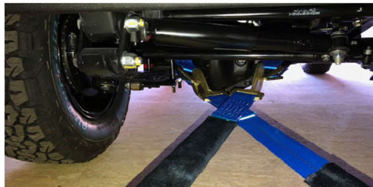
Figure 5. Straps to trailer tie downs
