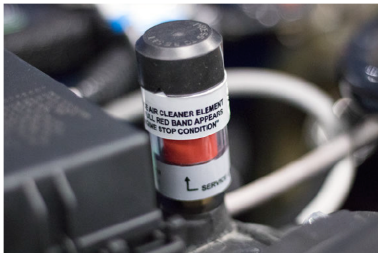
Figure 21. Air Filter Indicator
