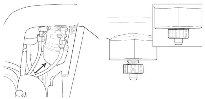
Figure 15. Fuel/ Water Separator Location
