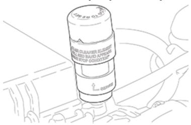
Figure 20. Air Filter Indicator
