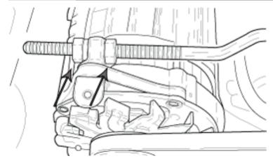
Figure 18. Alternator Adjustment Nut
