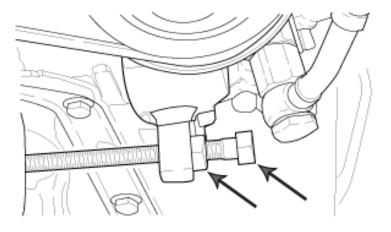
Figure 19. Power Steering Adjustment Nut
