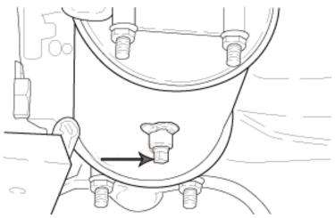
Figure 8. Spark Arrester Clean-Out Plug
