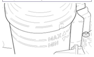
Figure 13. Power Steering Fluid Level
