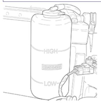
Figure 11. Coolant Overflow Bottle
