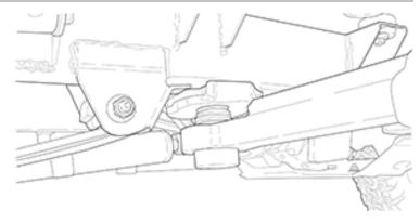
Figure 7. Rear Lifting Location
