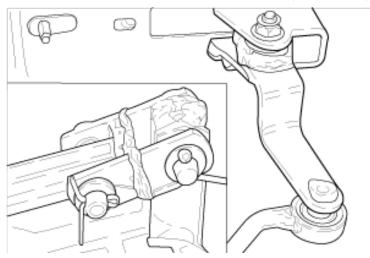
Figure 17. Shift Linkage Pivot Points
