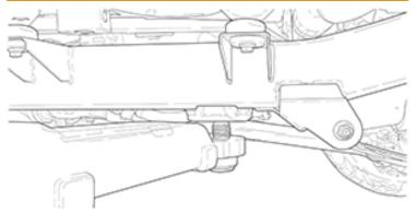
Figure 6. Front Lifting Location
