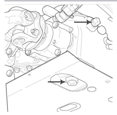
Figure 24. Transfer Drain Plug
