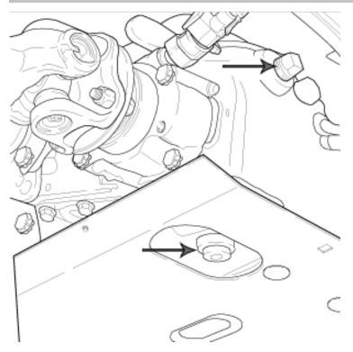
Figure 14. Transfer Case Oil Level Plug
