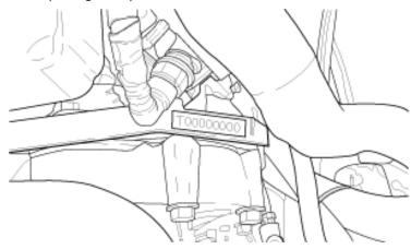
Figure 27. Engine Identification Number
