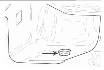
Figure 22. Oil Drain Plug
