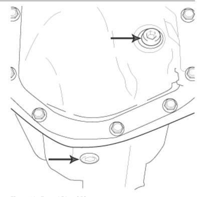
Figure 10. Front Oil Level Plugs
